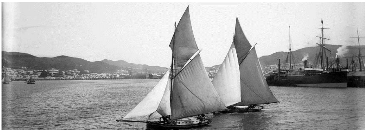
Xarifa , with her sensible rig, gets a nice lift and climbs to weather of a picturesque, but inefficiently rigged Thetis ca. 1880
