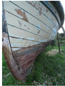
Mahoe in 2013 with later superstructure removed and seams reefed out ready for refastening
